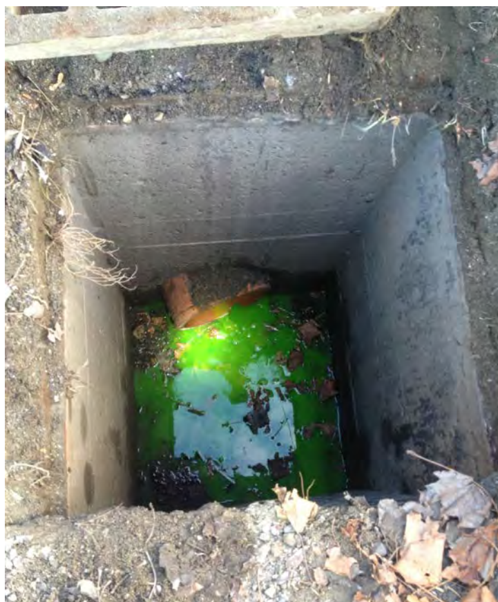
Figure 3. Dye flushed down a toilet at the elementary school appeared in catchbasin CB-C
